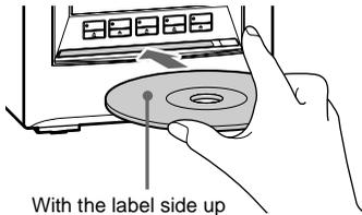
To load another disc, eject a disc or press one of the buttons (DISC 1 – 5) to select an empty compartment (it is not possible to select another compartment, when an 8 cm disc is loaded).
