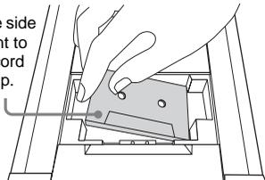
To remove the tape, lift up the tape from the side as shown in the illustration.
