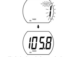
The display shows the frequency for about 10 seconds, and then returns to the current time.
