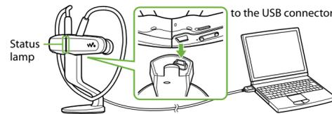
Charging starts. The status lamp blinks slowly during charging. When charging is completed, the status lamp will stop blinking and light dimly while the player is connected to the computer. For details about charging time and the battery duration, see "Specifications" on the reverse side.
