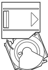
With the cut-away portion of the tray facing you, insert the right corner of the tray in the slot, then push in the left corner until it clicks.
