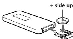
Replace the battery with a Sony CR2025 or Duracell DL-2025 lithium battery. Use of another battery may present a risk of fire or explosion.
