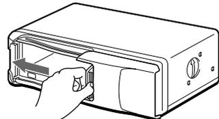
Use the supplied disc magazine or the disc magazine XA-250. The disc magazine XA-10B can not be used with this unit. If you use any other magazine, it may cause a malfunction.
