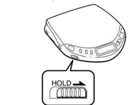
Slide HOLD in the direction of the arrow. The buttons are locked. when you press any button, "Hold" appears in the display.
