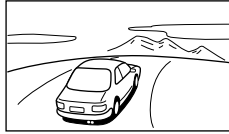
Wide-zoom screen An image with an aspect ratio of 4 to 3, with only the left and right sides of the image being enlarged to fill the screen.
