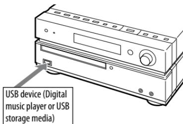
When USB cable connection is necessary, connect the USB cable supplied with the USB device to be connected.
