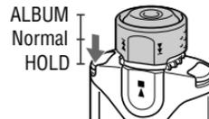
By pushing the Shuttle switch to the HOLD position, all operation buttons are disabled. If you press buttons while the HOLD function is activated, "HOLD" appears in the display.
